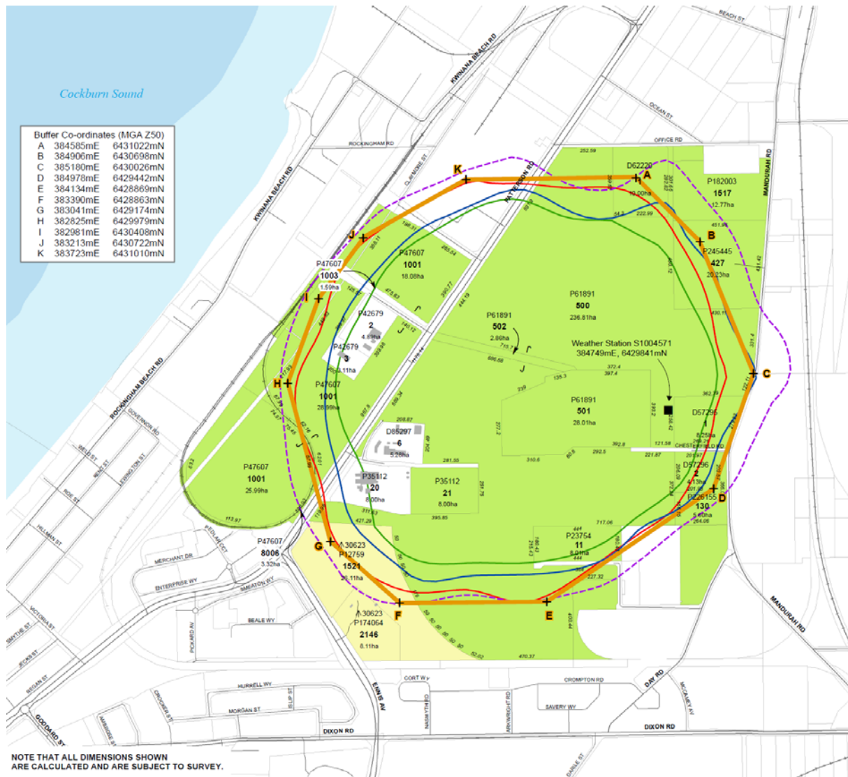
Figure 9. Predicted 7 OU Contour for Stages of East Rockingham WWTP, with Recommended Buffer Zone
